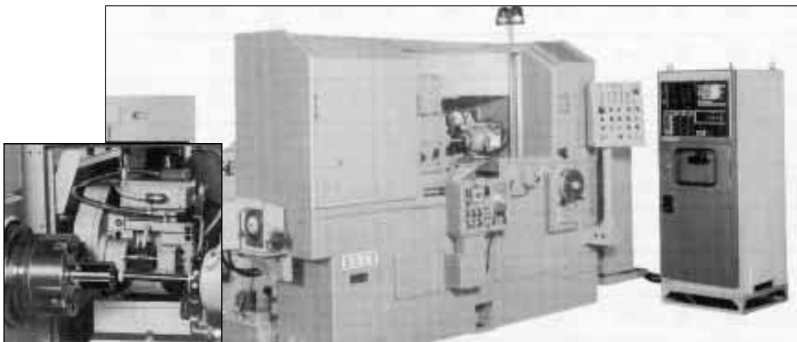
Grinding of Thread Groove of Nut
